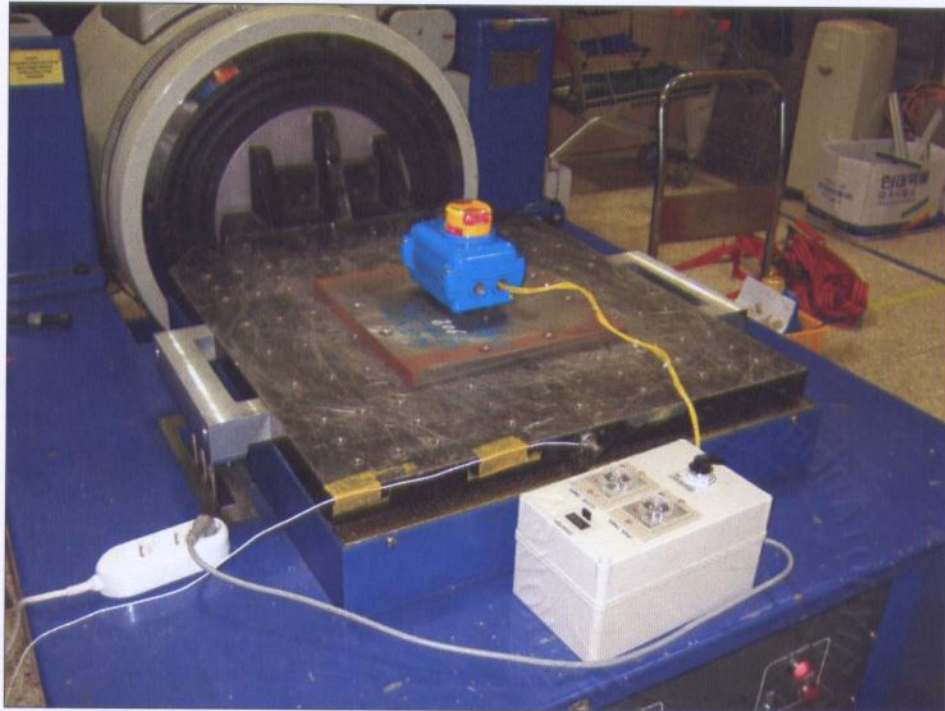
Figure 13. Test photo of Y axis vibration & mechanical shock test
