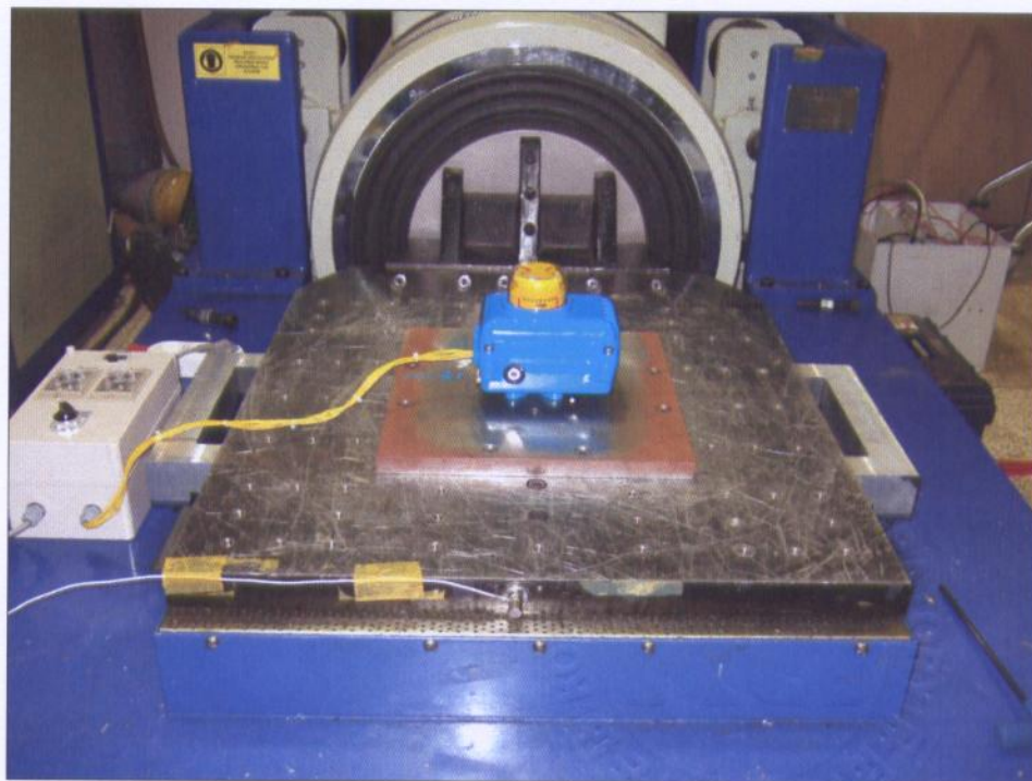
Figure 9. Test photo of X axis vibration & mechanical shock test
